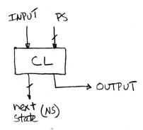
Given that we want to force a state transition on each clock cycle (remember that input bits are being applied one per clock cycle), we will put the combinational logic block in a loop with the state register as shown below:
