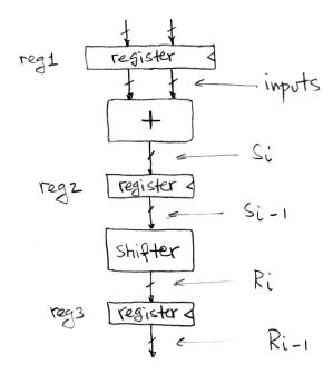
On each cycle, data moves from the output of reg1 through the adder to the input of reg2, or moves from the output of reg2 through the shifter to the input of reg3. Since the data no longer needs to move through both blocks on each cycle, the clock frequency can be increased. See the waveforms below:
