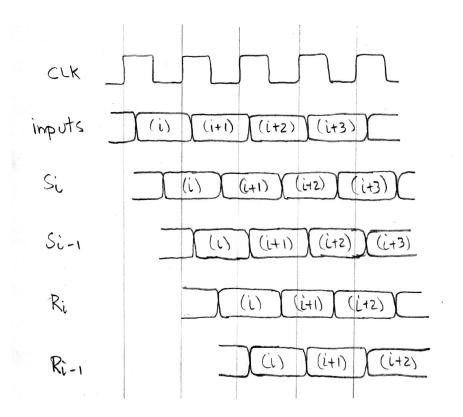
An interesting thing about this new circuit is that after the data moves through the adder and gets captured in reg2, on the next cycle when the data moves into the shifter, new data can simultaneously move into the adder, because it is free. Therefore new data values can be fed into the circuit on each clock cycle.
