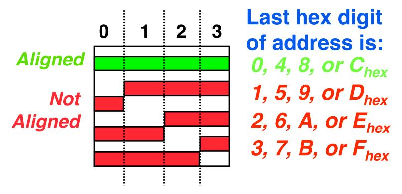
Called <u>Alignment</u>: objects must fall on address that is multiple of their size.
