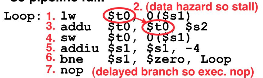
How many pipeline stages (clock cycles) per loop iteration to execute this code?
