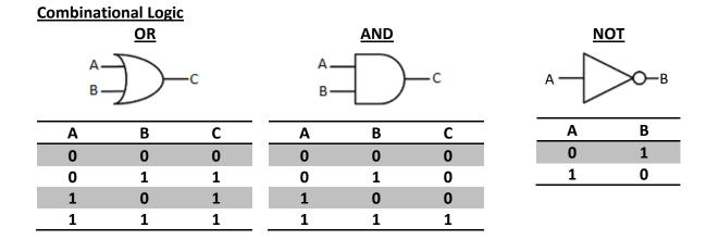
Using these above gates, create a NOR gate, a NAND gate, an XOR gate, and an XNOR gate.
