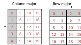
How a 4x5 Matrix is stored in memory, red numbers are memory addresses
