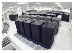
BlueGene/L – IBM/DOE Rochester, United States 32768 Processors, 70.72 Tflops/sec 0.7 GHz PowerPC 440
