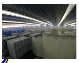
Earth Simulator – Earth Simulator Ctr. Yokohama, Japan 5120 Processors, 35.86 Tflops/sec SX6 Vector
