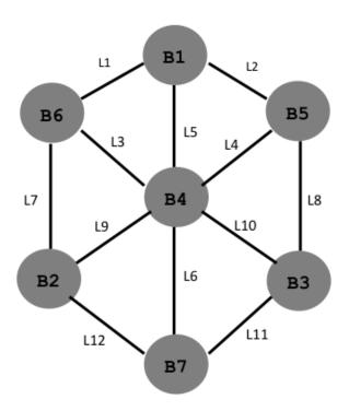
Reminder: (i) the root is the bridge with the lowest ID, and (ii) when there is more than one shortest path to the root, the path whose first hop goes through the bridge with the lower ID is chosen. Also, each link is considered to have a length of one when computing path lengths.
