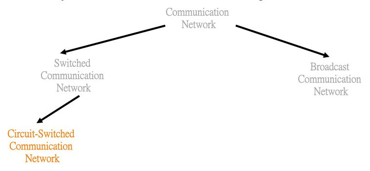
Communication networks can be classified based on the way in which the nodes exchange information:
