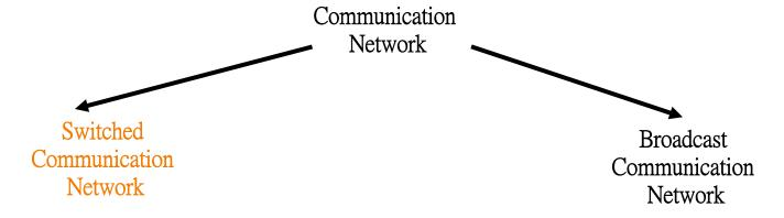
The term "switched" means that communication is directed to specific destinations
